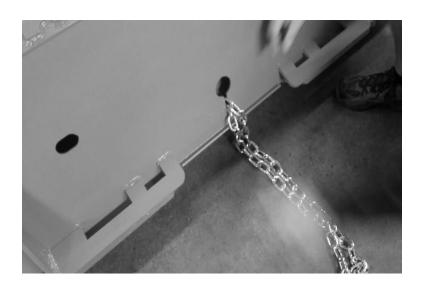
Step 3: Take the loose end of the chain and secure it to the Brush Cutter.
