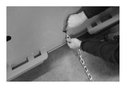
Step 2: Using one end of safety chain, drop number of desired links into link hole.
