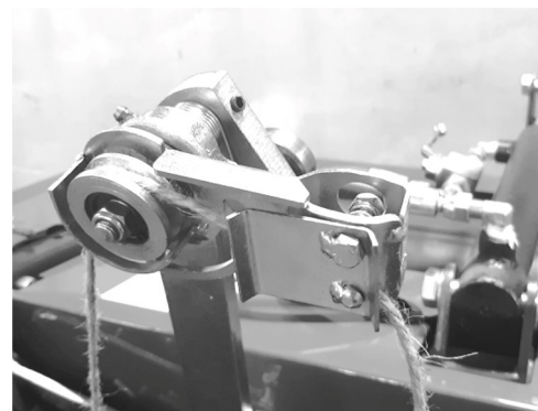
Twine Tensioner #2 (end of binding arm)
