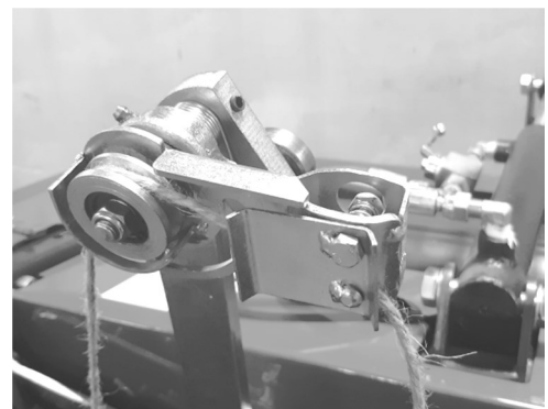
Twine Tensioner 2 (end of binding arm)
