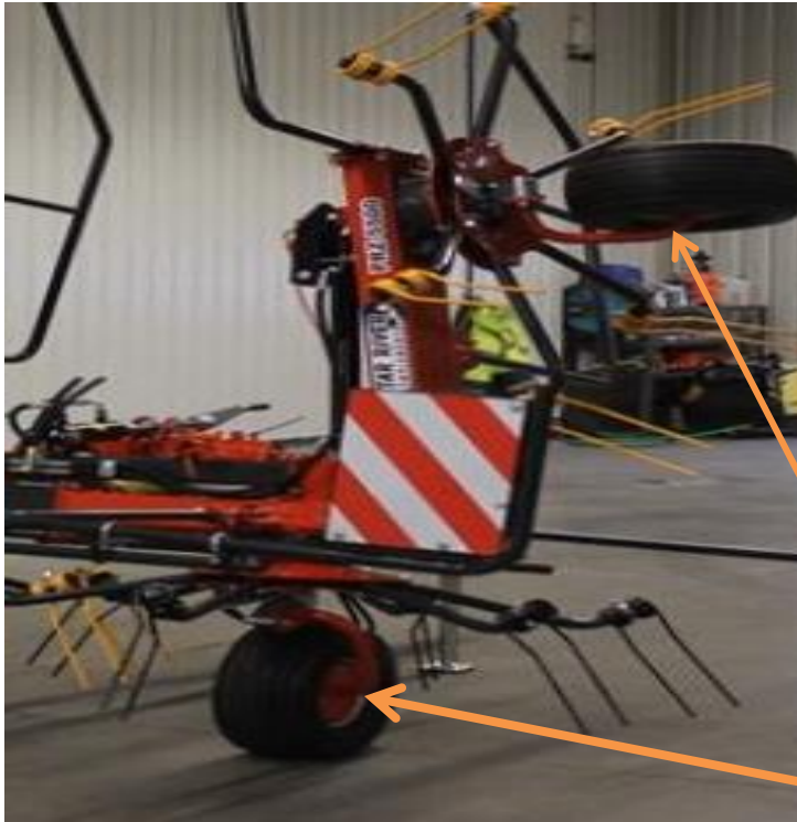
Hub Covers on the inside of outer and inner baskets to protect spindles
