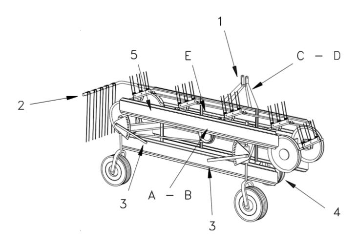
1. Three Point Linkage, 2. Hay Stopper, 3. Adjustment Bar, 4. Third Wheel, 5. Guards
