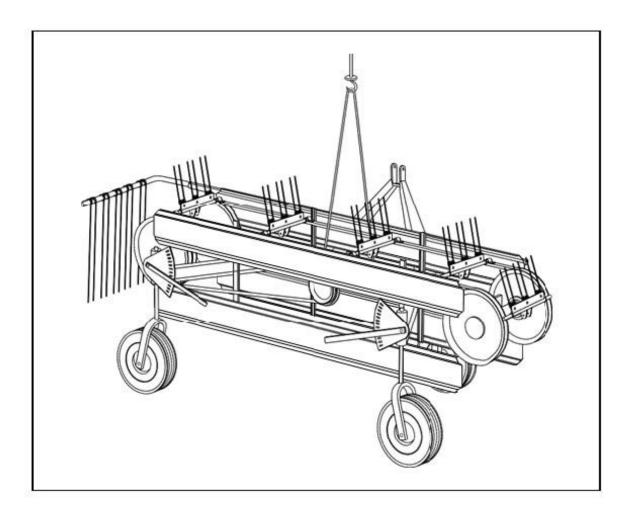
To load the belt-type windrower with a hoist, insert a belt straddling the power take off and the frame, fix the two ends of the belt to the crane hook.
